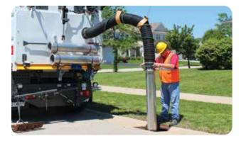
The combination Elgin Whirlwind1 sweeper with wandering hose option provides a cost-effective tool to facilitate storm water management.
