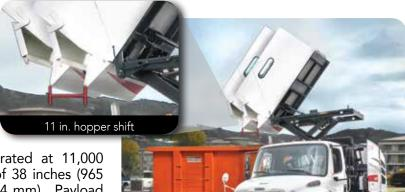
A unitized, twin-cylinder, double scissors lift rated at 11,000 lbs (4,990 kg) unloads material at a minimum of 38 inches (965 mm) and a maximum of 11 feet, 2 inches (3,404 mm). Payload capacity is 10,000 lbs (4,536 kg) per load. An 11 inch (279 mm) side shift allows material to be unloaded into the center of a truck or container for cleaner dumping. A full hopper can dump and retract in 20 seconds for short intervals and up to 70 seconds at top height.
