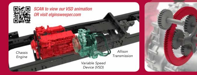
The VSD replaces the diesel auxiliary engine, eliminates a complex aftertreatment system, and untimely regenerations. It's simple to operate, and carries a three year warranty.
