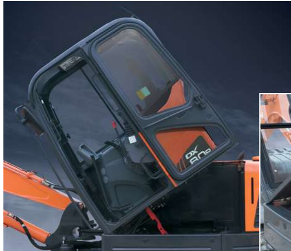
Tilting cabin for easy maintenance
