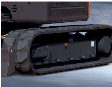
Rubber tracks The rubber tracks not only offer greater non-slip and grip capabilities but are also less harmful to pavements and road surfaces in urban environments than conventional steel shoes. These rubber tracks can be easily installed or removed with the idler, sprocket and other main parts.
