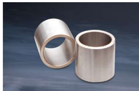
Bushing A highly lubricated metal (sintered bushing) is used for the boom, arm and bucket pivots in order to extend the greasing intervals to upto 250 hours and increase the bush life.
