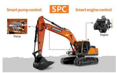
SPC is a predictive powertrain control system, which automatically identifies working mode and adjusts engine RPM to supply proper pump torque. SPC relieves the driver's workload and contributes to a fuel-efficient working style. Raising the pump torque up to maximize when productivity and power is needed. Lowering the pump torque down to reduce unnecessary fuel consumption when fuel efficiency is needed.
