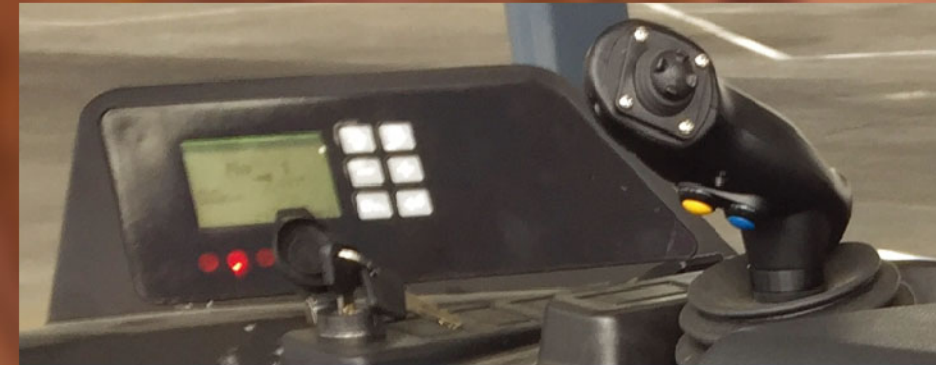
ZAPI smart display & multi-function joystick
